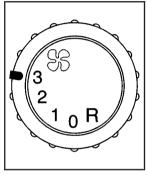
To adjust the airflow speed, turn the fan knob (driver override switch), located on the floor console to 1, 2 or 3. The rear mode and temperature positions now mimic the front control system mode and passenger side temperature.
